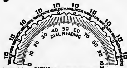
KARAS ORTHOMETRIC CONDENSER Arrangement of Wavelengths on Dial
